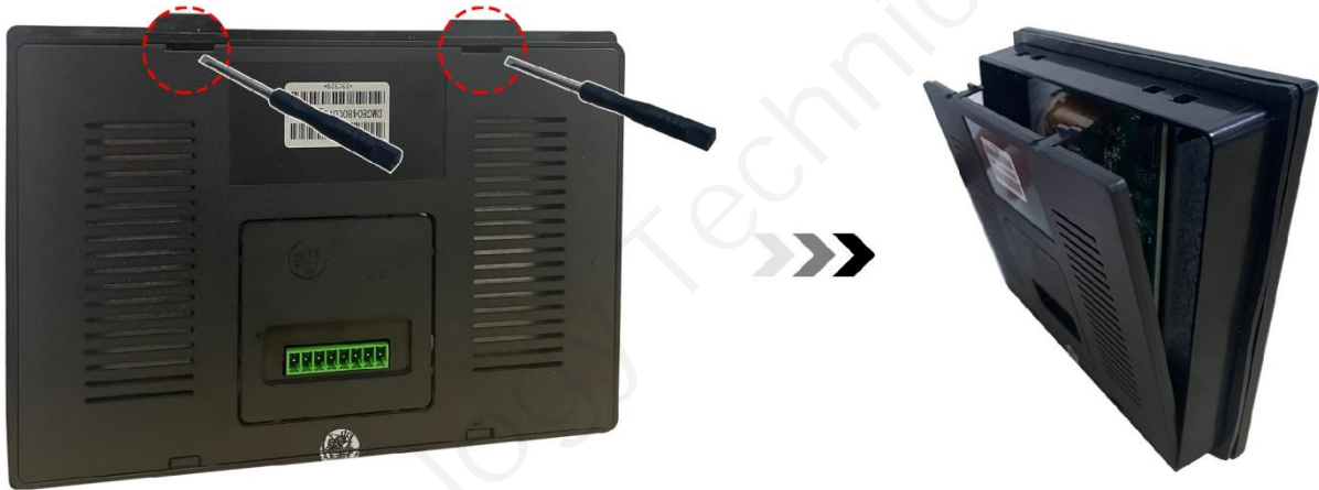
Press the buckle with a slotted screwdriver or similar tool and disassemble it outward
