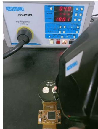
4.1 Electrostatic discharge test
