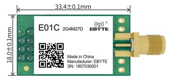
transmitting power reach 500mW, and the communication stability is greatly improved compared with the products without power amplifier and low-noise amplifier, and the industrial-grade high-precision 16MHz crystal is used.
