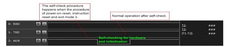
Timing Sequence Diagram of AUX when self-check
