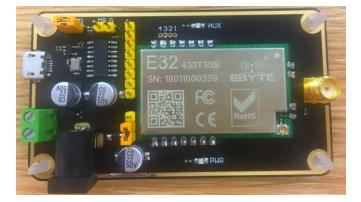
As shown in the figure, plug in the jumper (select 5V power supply, mode 1). For details, please refer to the corresponding serial port module manual.
