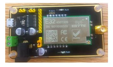
As shown in the figure, plug in the jumper (select 5V power supply, mode 3). For details, please refer to the corresponding serial port module manual.
