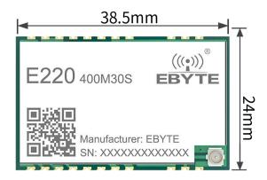
performance and communication distance have been improved, further opening the gap with FSK and GFSK modulation products. The product can cover an ultra-wide frequency range of 410~493MHz.
