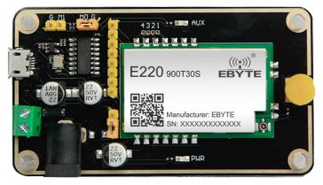
As shown in the figure, plug in the jumper (select 5V power supply, mode 2). For details, please refer to the corresponding serial port module manual.
