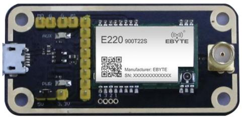
As shown in the figure, plug in the jumper (select 5V power supply, mode 3). For details, please refer to the corresponding serial port module manual.
