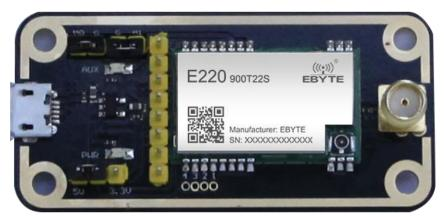
As shown in the figure, plug in the jumper (select 5V power supply, mode 0), both E22-900TBL-01 are configured as the same, open the corresponding serial port, you can send and receive data, and you can observe that the AUX light of the backplane flashes.
