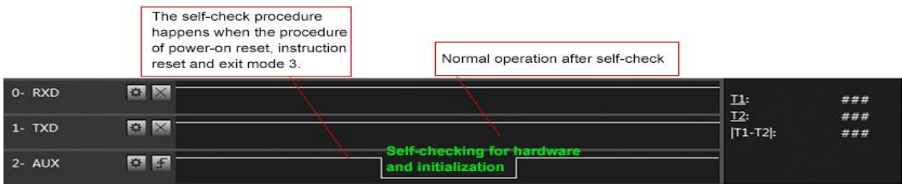
Timing Sequence Diagram of AUX when self-check
