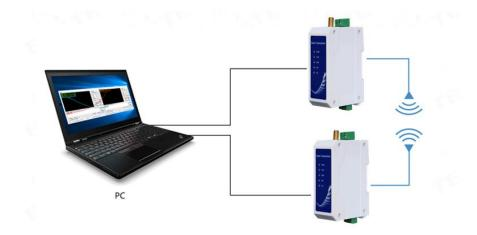
Start two serial port debugging assistants, select the serial port baud rate as 9600bps (default), and check the mode as 8N1, then the serial port transparent transmission can be realized.;
