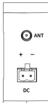
E95-DTU (900SLxx-485) can be powered by 8~28V (DC) power supply, and the wiring port is connected by wiring terminal (2 Pin).
