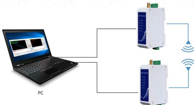
Start two serial port debugging assistants, select the serial port baud rate as 9600bps (default), and check the mode as 8N1, then the serial port transparent transmission can be realized.;
