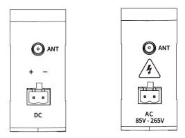
E95/E96-DTU (400SLxxx) can be powered by  $8\sim28V(DC)/85\sim265V(AC)$  power supply, and the wiring terminal is connected by terminal (2 Pin).
