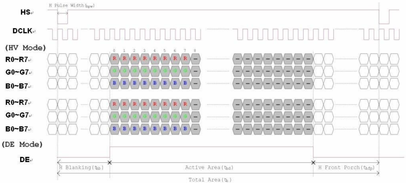
Horizontal input timing diagram
