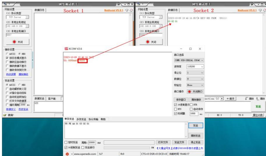
3. The data sent by the serial port is arbitrary data, and the data will be transmitted to two Sockets.
