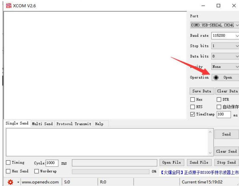
(5) Data transmission test, the serial port assistant (serial port side) sends test data, and the network debugging assistant (network side) receives the test data. The network debugging assistant (network side) sends test data, and the serial port assistant (serial port side) receives the test data. Realize duplex communication (that is, two-way data sending and receiving from local to network).
