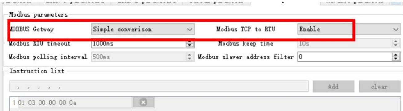
After turning on simple protocol conversion, TCP to RTU conversion is enabled: Modbus RTU protocol and Modbus TCP protocol are converted to each other, and non-Modbus data (R TU/TCP ) is directly discarded.
