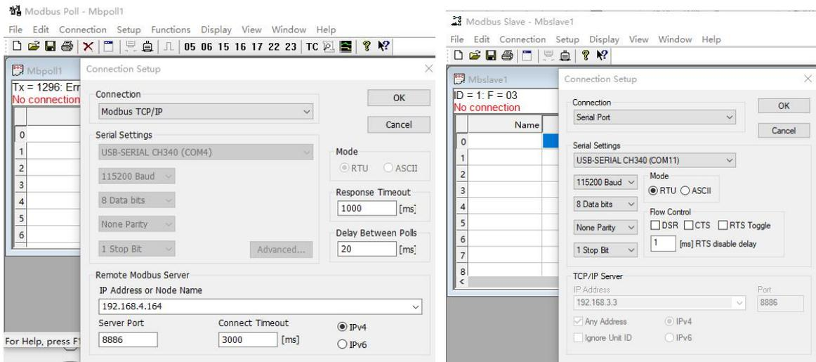
Software register reading and simulation configuration:
