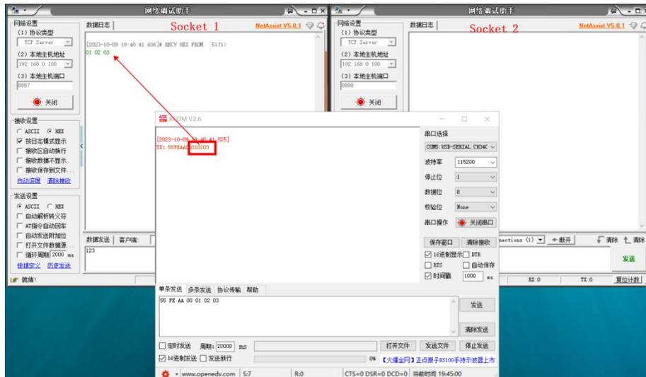
2. The serial port sends data if the data header is 55 FE AA 01, which means it meets the requirements, that is, 55 FE AA 01+data, then the data will only be transmitted to Socket 2, and the received content only contains data, without the data header;
