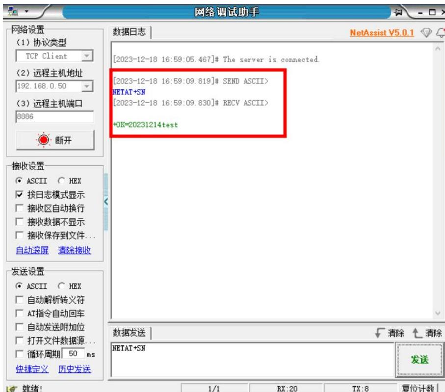
If the current AT command header is NETAT, you can send commands through the network to query and configure parameters after the link is successfully connected. If you send
