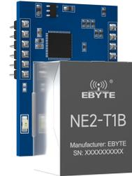
The product comes with an RJ45 interface, which is compact and easy to use (also known as the "super network port"). The product comes with RJ45 interface and pin packaging. It can meet the networking functions of various TTL level serial devices and MCUs . It adopts a small size design of 34.86×22×24mm, which is convenient for users to integrate into the system.
