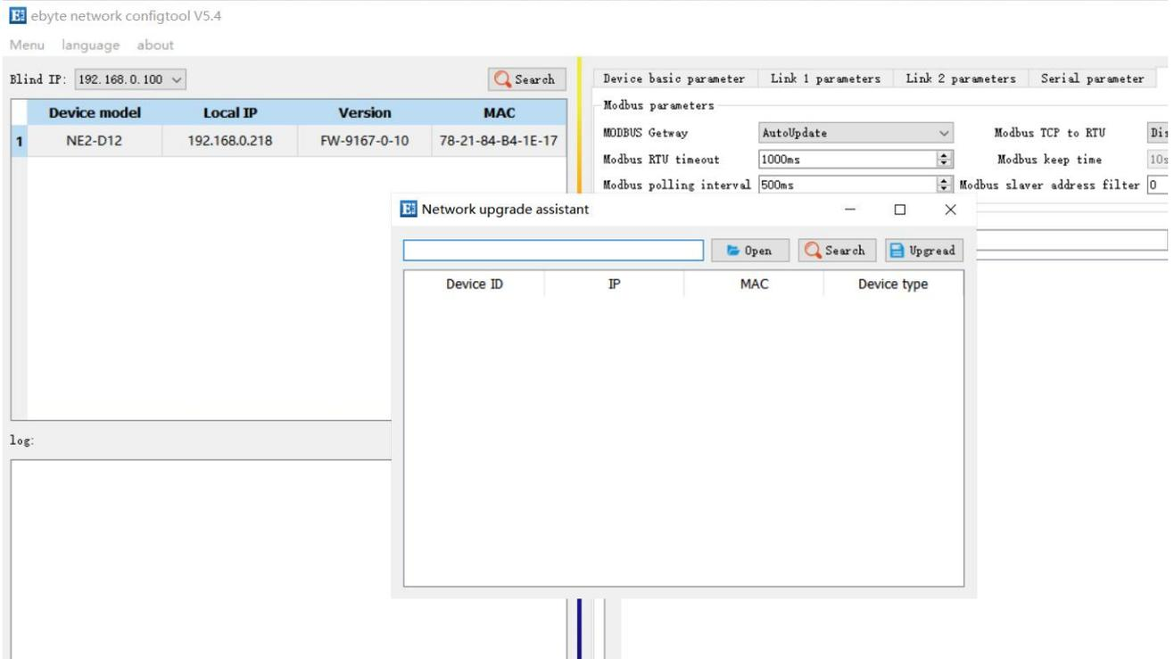
Step 3: In the pop-up "Device Network Upgrade Assistant" dialog box, click "Search for Device" (the computer and the device should be in the same network segment), and click "Stop Search" after searching for the device;
