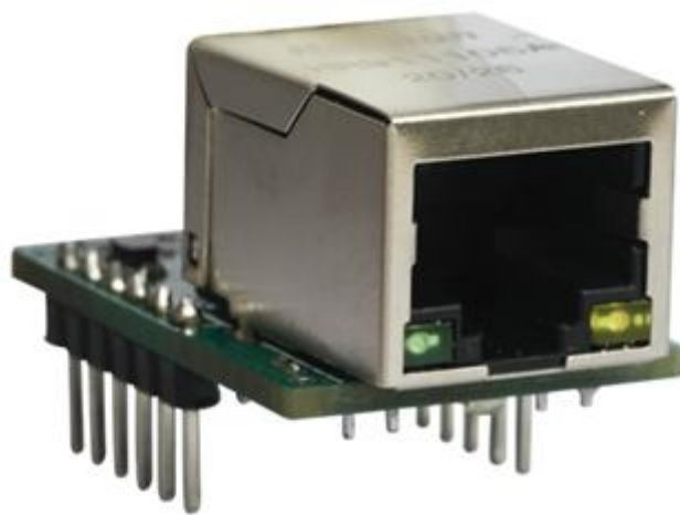
Network port forward installation NT1-B
