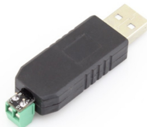
RS485 serial to USB cable
