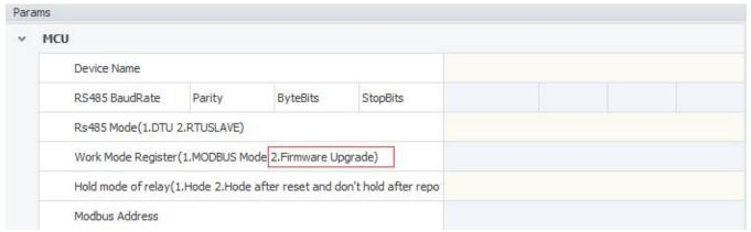
Step 2: After finishing downloading, device will upgrade firmware automatically and LED WORK will fast blink.
