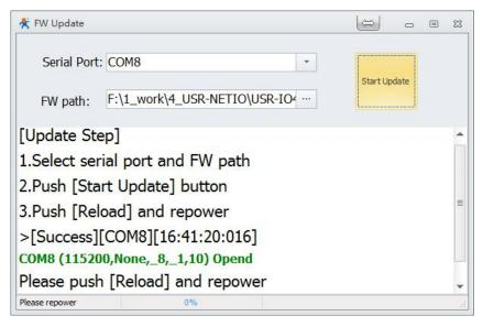
Step 3: Press 'Reload' button to restart device, LED WORK will fast blink which means device start upgrading.
