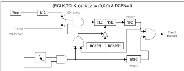
Figure 14-5 16-Bit Auto-reload Mode, Counting Up
