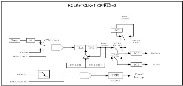
Figure 14-7 Baud Rate Generator Mode
