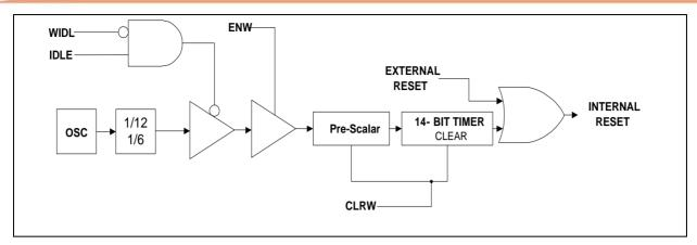
Figure 15-1 Watchdog Timer Block Diagram
