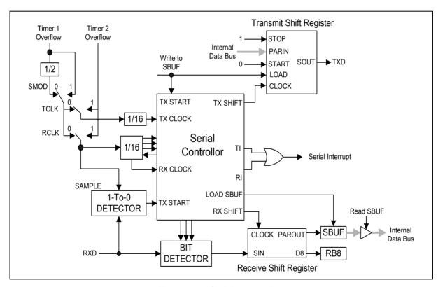
Figure 16–2 Serial port mode 1
