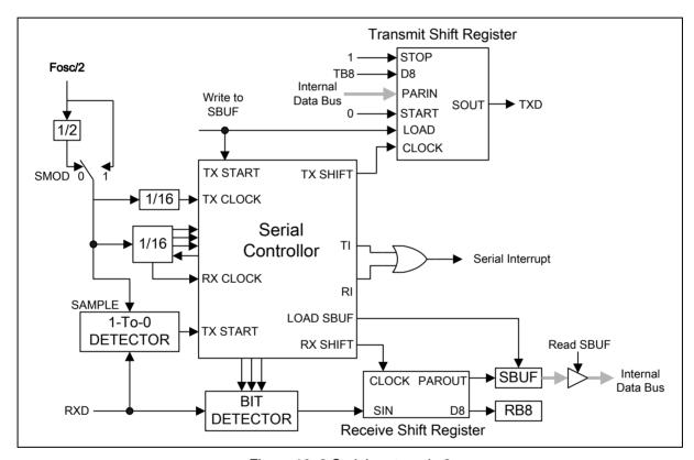
Figure 16-3 Serial port mode 2
