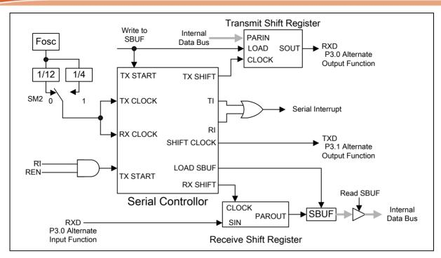
Figure 16-1 Serial port mode 0
