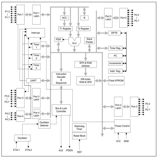
Figure 6-1 W78E054D/W78E052D Block Diagram
