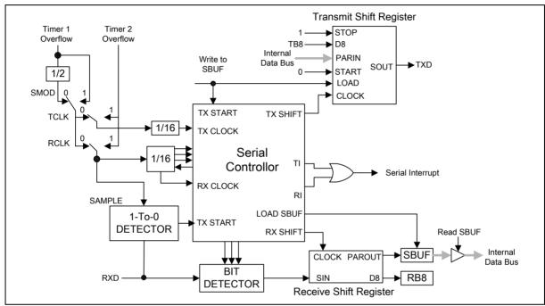
Figure 16–4 Serial port mode 3
