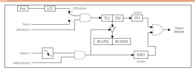
Figure 14-4 16-Bit Capture Mode
