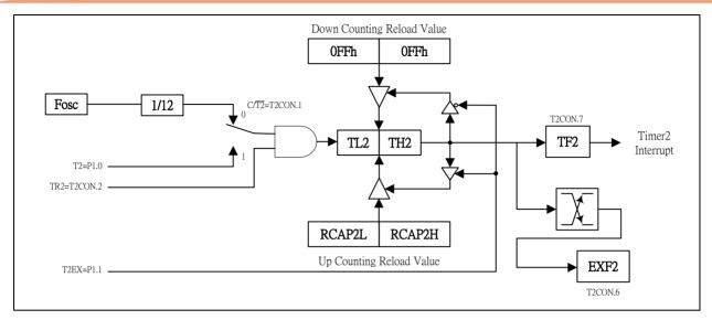
Figure 14-6 16-Bit Auto-reload Mode, Counting Up
