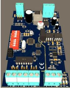
The IO modules are mounted on DIN rail mountable enclosure. There is LED indication for Power, Modbus TX/RX
