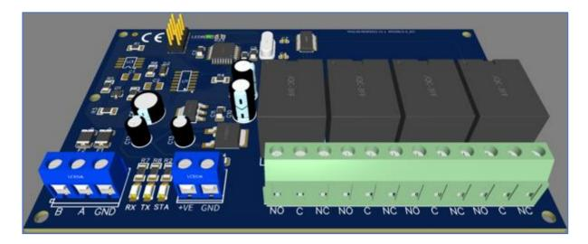
The IO modules are mounted on DIN rail mountable casing and will also have a top acrylic safety cover on top for safety.
