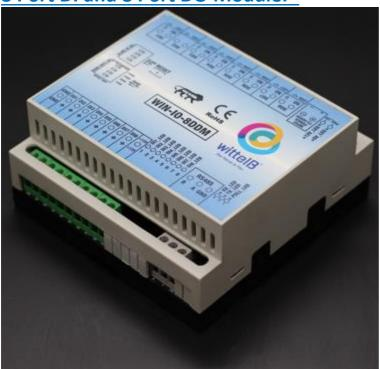
The IO modules are mounted on DIN rail mountable casing and with exposed connectors and LED indicators. The DIP switch for Slave ID and Baud rate are placed inside the enclosure.
