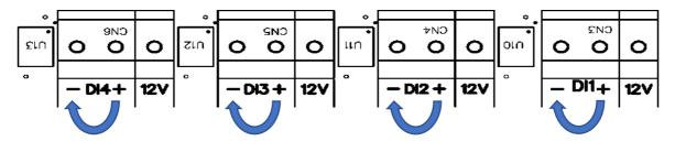
For Digital Input with Potential (3V to 30V) Contact + Common GND terminal should be connected on the Board, e.g DI1 +ve terminal and GND pin.
