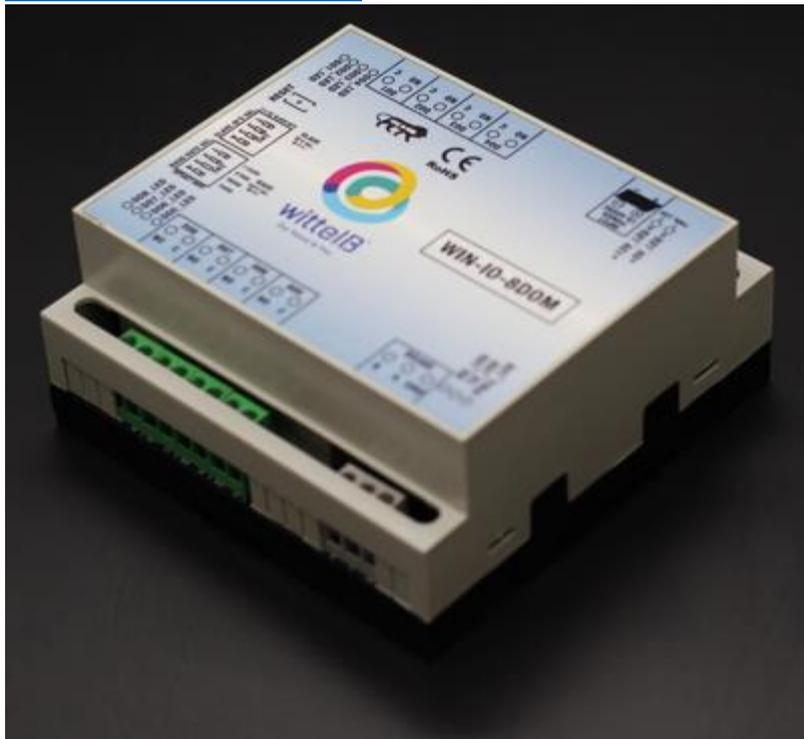
The IO modules are mounted on DIN rail mountable casing and with exposed connectors and LED indicators. The DIP switch for Slave ID and Baud rate are placed inside the enclosure.
