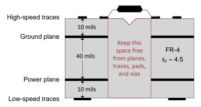
Figure 19. Recommended Layer Stack
