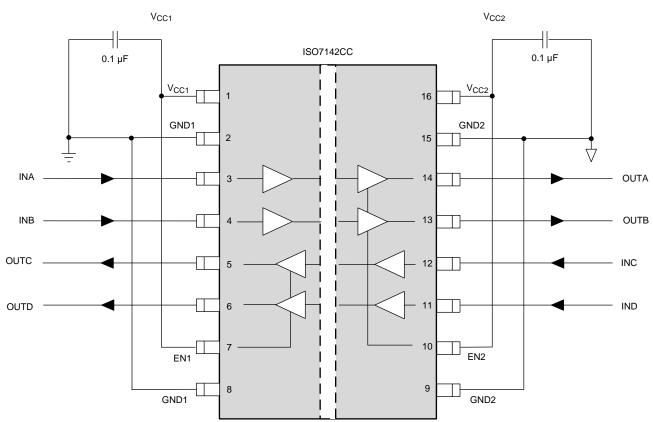
Figure 15. Typical ISO7142CC Circuit Hook-up
