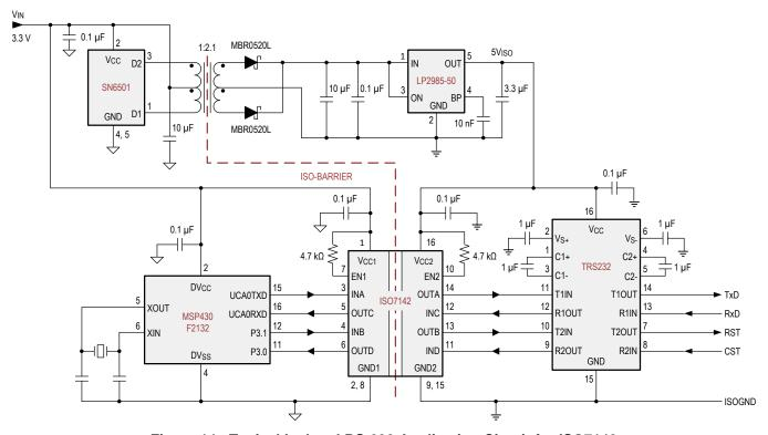
Figure 14. Typical Isolated RS-232 Application Circuit for ISO7142
