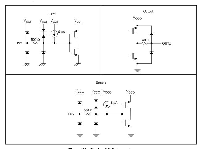
Figure 13. Device I/O Schematics
