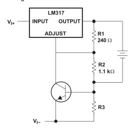
Figure 21. Current-Limited 6-V Charger Circuit
