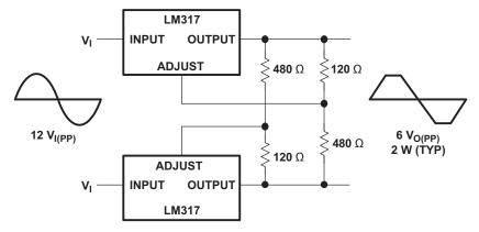
Figure 20. AC Voltage-Regulator Circuit
