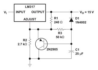
Figure 19. Slow Turn-On 15-V Regulator Circuit
