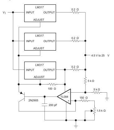
Figure 22. Adjustable 4-A Regulator Circuit
