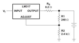
Figure 17. Battery-Charger Circuit
