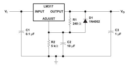
Figure 13. Adjustable Regulator Circuit with Improved Ripple Rejection
