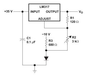
Figure 12. 0-V to 30-V Regulator Circuit
