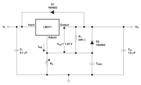
Figure 9. Adjustable Voltage Regulator
