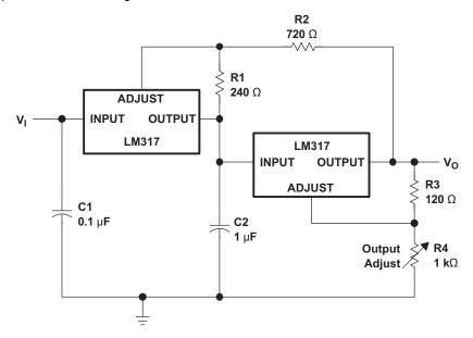
Figure 15. Tracking Preregulator Circuit
