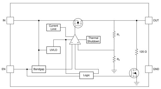
$R_2$  = 550 k $\Omega$ ,  $R_1$  = adjustable.
