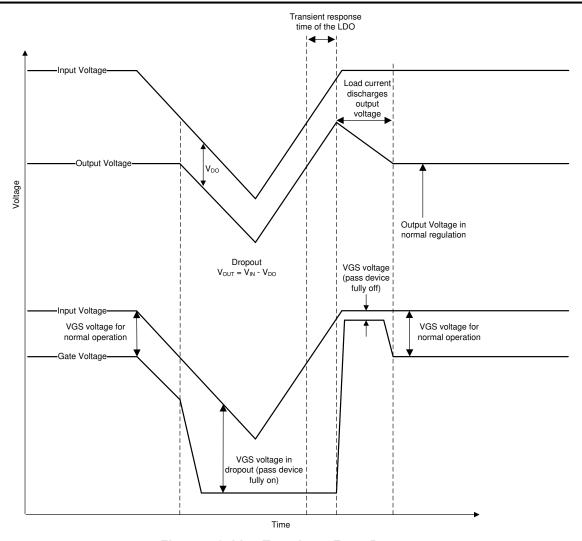
Figure 7-2. Line Transients From Dropout
