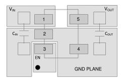
Represents via used for application specific connections
