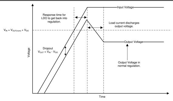
Figure 7-1. Start-Up Into Dropout
