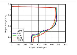
Figure 5-26. 3.3-V Foldback Current Limit, V<sub>OUT</sub> vs I<sub>OUT</sub>
